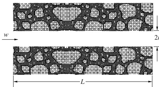
Fig. 3. Schematics of macroregular (planar) packing of adsorbent sheets in an adsorber. Gas is filtered between sheets in the Poiseuille flow.
