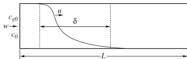
Fig. 2. Schematic of the adsorption front.
