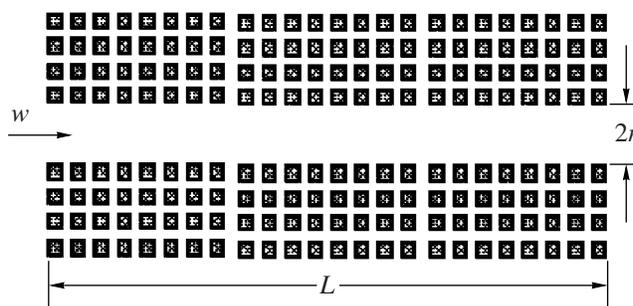
Fig. 4. Schematics of macro- and microregular adsorbent packing in a sheet. Squares, zeolite crystallite; gaps between squares, transport nanopore system. Gas is filtered between sheets in the Poiseuille flow.
